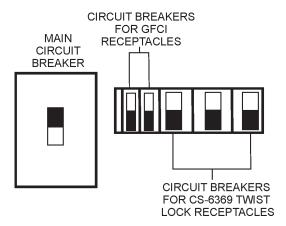
Figure 57. Main, Aux. and GFCl Circuit Breakers (ON)
